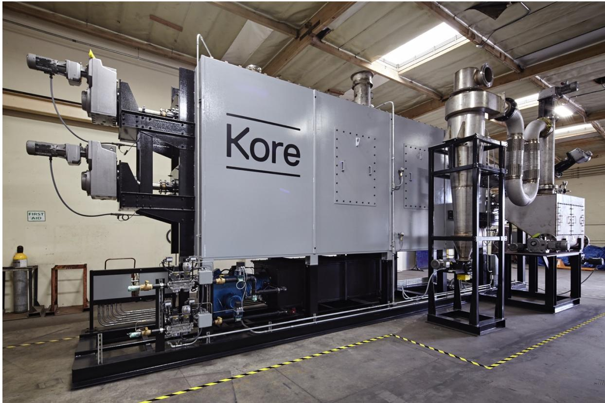
Kore Infrastructure's pyrolyzer, a key piece of the company's waste-to-energy solution that sustainably converts treated sewage sludge into renewable natural gas
